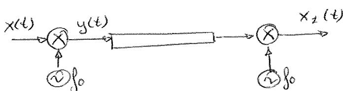
$$\begin{aligned} x_1(t) &= y(t) \cdot \cos(2\pi f_0 t) = A \cdot x(t) \cdot \cos^2(2\pi f_0 t) = A \cdot x(t) \frac{1 + \cos(4\pi f_0 t)}{2} \\ &= \frac{A}{2} x(t) + \frac{A}{2} x(t) \cdot \cos(4\pi f_0 t) \end{aligned}$$
