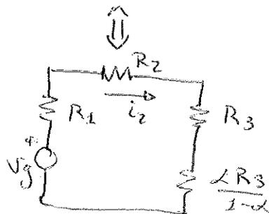
$$i_2 = \frac{V_g}{R_1 + R_2 + R_3 + \frac{R_3 \alpha}{1-\alpha}}$$
