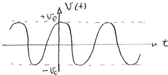
$$V(t) = V_0 \cos(\omega t + \varphi)$$
