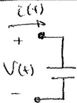
$$\left. \begin{aligned} p(t) &= V(t) i(t) \\ i(t) &= C \frac{dV}{dt} \end{aligned} \right\} \begin{aligned} p(t) &= C V(t) \frac{dV}{dt} = \frac{d}{dt} \left[ \frac{C}{2} V^2(t) \right] \end{aligned}$$
