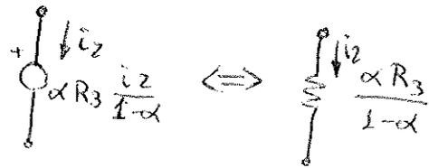
$$V = I R = \alpha R_3 \frac{i_2}{1-\alpha} ; R = \frac{V}{I} = \frac{\alpha R_3}{1-\alpha}$$
