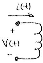
$$\left. \begin{aligned} p(t) &= V(t) \cdot i(t) \\ V(t) &= L \cdot \frac{di}{dt} \end{aligned} \right\} \begin{aligned} p(t) &= L i(t) \frac{di}{dt} = \frac{d}{dt} \left[ \frac{L}{2} i^2(t) \right] \\ p(t) &= \frac{dW}{dt} \end{aligned}$$
