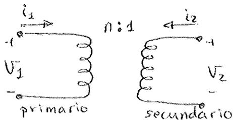
$$\begin{aligned} V_1 &= n V_2 \\ i_2 &= -n i_1 \end{aligned}$$
