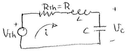
$$V_{Th} = RC \frac{dV_c}{dt} + LC \frac{d^2V_c}{dt^2} + V_c(t)$$
