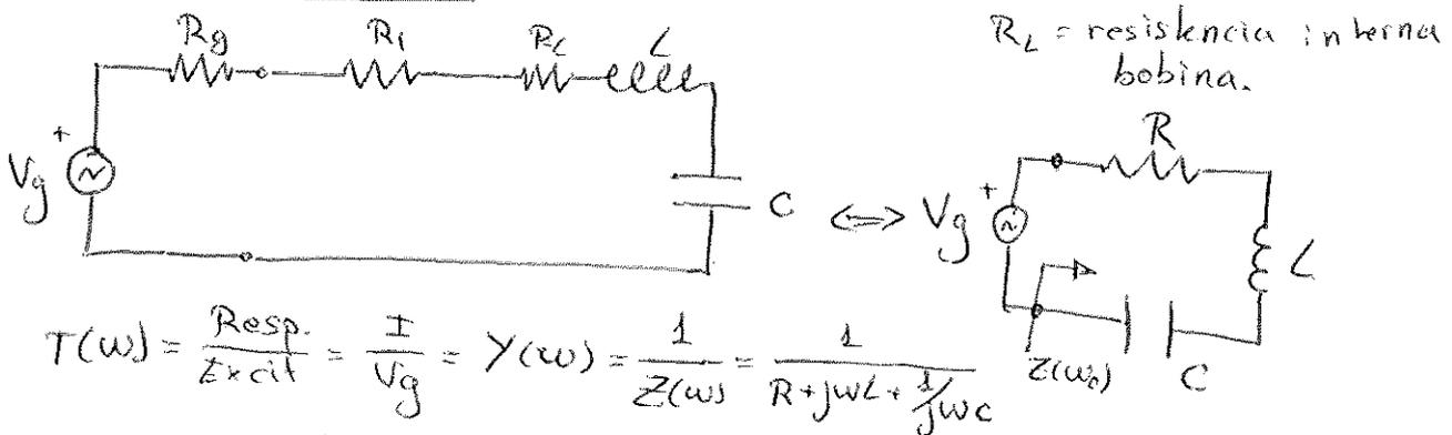
$$T(\omega) = \frac{Resp.}{Z_{excit}} = \frac{I}{V_g} = Y(\omega) = \frac{1}{Z(\omega)} = \frac{1}{R + j\omega L + \frac{1}{j\omega C}}$$
