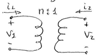
$$V_1 = n V_2$$
