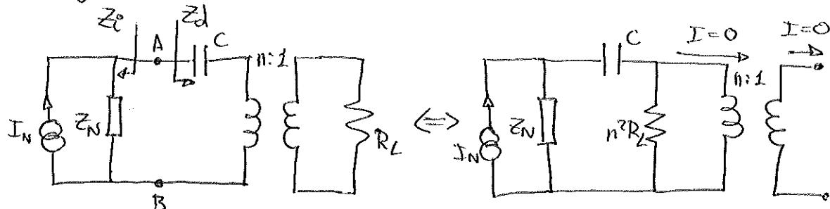
$$Z_i = Z_N = Z_{eqAB} = R_g \parallel j\omega L_2 = \frac{R_g j\omega L_2}{R_g + j\omega L_2} = \frac{\omega^2 L_2^2 R_g}{R_g^2 + \omega^2 L_2^2} + j \frac{\omega L_2 R_g}{R_g^2 + \omega^2 L_2^2}$$
