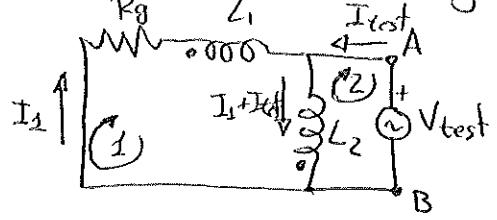
$$\begin{aligned} \text{malla 1: } & I_1 R_g + I_1 j\omega L_1 + (I_1 + I_{\text{test}}) j\omega L_2 = \\ & = (I_1 + I_{\text{test}}) j\omega M_{12} + I_1 j\omega M_{12} \quad \} \\ \text{malla 2: } & V_{\text{test}} + (I_1) j\omega M_{12} = (I_1 + I_{\text{test}}) j\omega L_2 \end{aligned}$$
