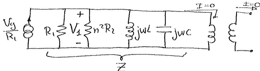
$$V_1 = Z \frac{V_g}{R_1} \quad \left. \begin{array}{l} \\ \end{array} \right\} V_1 = \frac{R}{R_1} V_g$$
