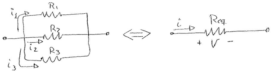
$$\frac{1}{R_{eq}} = \frac{1}{R_1} + \frac{1}{R_2} + \frac{1}{R_3} \quad ; \quad i = i_1 + i_2 + i_3 \quad ; \quad V = V_1 = V_2 = V_3$$
