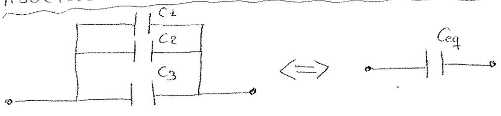
$$C_{eq} = C_1 + C_2 + C_3$$
