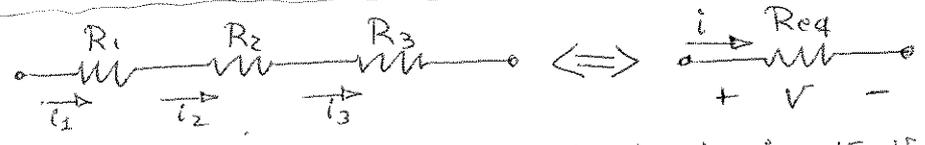
$$R_{eq} = R_1 + R_2 + R_3 \quad ; \quad i_1 = i_2 = i_3 = i \quad ; \quad V = V_1 + V_2 + V_3$$
