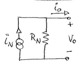
$$V_{TH} = R_{TH} \cdot i_N = R_N \cdot i_N \Rightarrow R_{TH} = R_N$$
