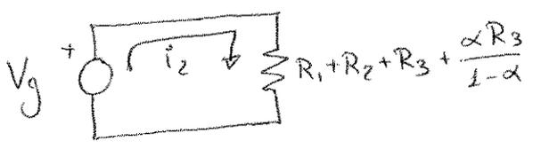
$$i_2 = \frac{V_g}{R_1 + R_2 + R_3 + \frac{\alpha R_3}{1-\alpha}}$$
