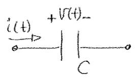
$$C \text{ (capacidad)} = \frac{Q}{V} \quad (\text{Faradios, F})$$
