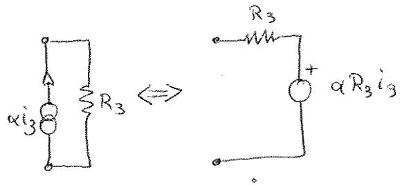
$$\alpha R_3 i_3 = \alpha R_3 \frac{i_2}{1-\alpha}$$
