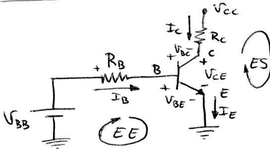
EE:  $V_{BB} - I_B R_B - V_{BE} = 0$
