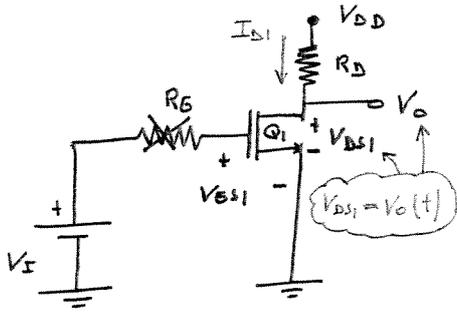
$V_{GS1} = V_i = 5V \geq V_T \Rightarrow$  NO ESTÁ EN CORTE
