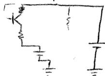
$$ES: V_{CE}^{sat} + I_E R_D + V_{CE} + I_C R_B - V_{CC} = 0$$
