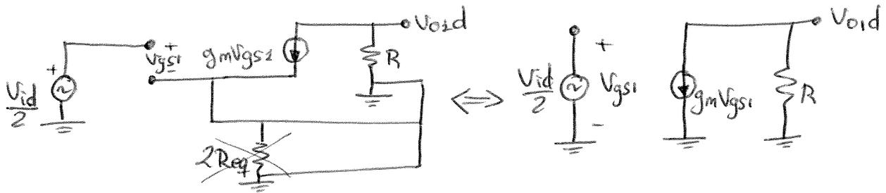
$$\left. \begin{aligned} V_{oid} &= -g_m V_{gs1} \cdot R \\ V_{gs1} &= \frac{V_{id}}{2} \end{aligned} \right\} \begin{aligned} V_{oid} &= -g_m \frac{V_{id}}{2} \cdot R \\ V_{oid} &= -g_m \frac{V_{id}}{2} R \end{aligned} \Rightarrow \boxed{A_d = \frac{V_{oid}}{V_{i1}} = \frac{-g_m R}{2} = -1}$$
