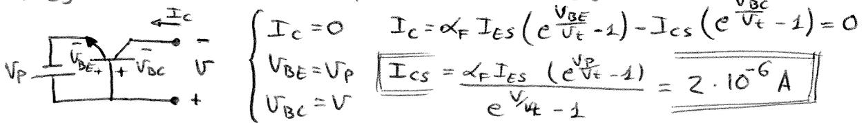
$$\begin{cases} I_C = 0 & I_C = \alpha_F I_{ES} (e^{\frac{V_{BE}}{V_t}} - 1) - I_{CS} (e^{\frac{V_{BC}}{V_t}} - 1) = 0 \\ V_{BE} = V_P & \boxed{I_{CS} = \frac{\alpha_F I_{ES} (e^{\frac{V_P}{V_t}} - 1)}{e^{\frac{V}{V_t}} - 1} = 2 \cdot 10^{-6} \text{ A}} \\ V_{BC} = V \end{cases}$$
