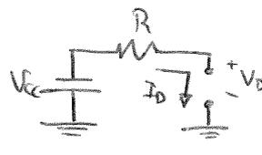
$$\begin{aligned} I_D(t) &= 0 \quad (t < 0) \\ V_D(t) &= -V_{CC} = -5 \text{ V} \end{aligned}$$
