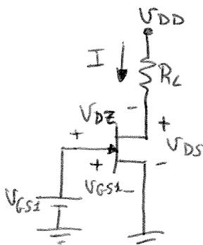
\*  $i_D = I = I_{DSS} \left(1 - \frac{V_{GS1}}{V_T}\right)^2 \Rightarrow V_{GS1} = \left(1 \pm \sqrt{\frac{I}{I_{DSS}}}\right) V_T \Rightarrow$
