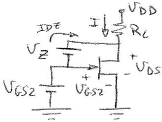
\*  $V_{GS2} = V_{DS} - V_Z = 5 - 8 = -3V \geq V_T$  (ok)
