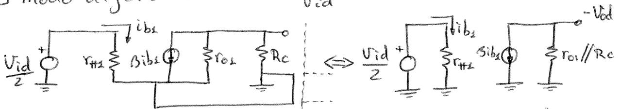
$$\left. \begin{aligned} -V_{od} &= -\beta i_{b1} (r_{o1} // R_c) \\ V_{id} &= 2 i_{b1} r_{\pi 1} \end{aligned} \right\} \boxed{A_d = \frac{V_{od}}{V_{id}} = \frac{\beta (r_{o1} // R_c)}{2 r_{\pi 1}} = 167}$$
