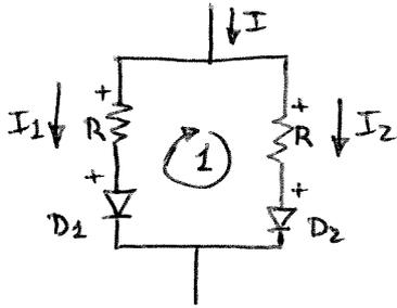
$$R = \frac{V_{D1} - V_{D2}}{I_2 - I_1} = \frac{0'617 - 0'672}{0'476\text{mA} - 0'524\text{mA}} = \underline{\underline{1'15\text{ K}\Omega}}$$
