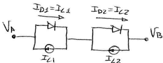
$$V_{AB} = V_{D1} + V_{D2}$$
