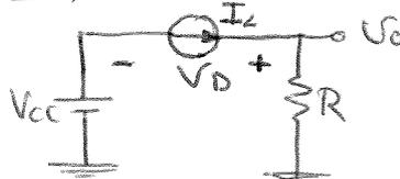
$$V_D = V_o - V_{CC} = 1 - 5 \leq V_\gamma \text{ (o.k.)}$$
