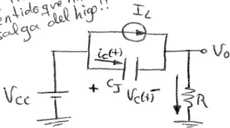
$$V_0(t) = (I_L + i_c)R = I_L R + C_J R \frac{\partial V_c(t)}{\partial t} = I_L R + C_J R \frac{\partial}{\partial t} (V_{cc} - V_0(t))$$
