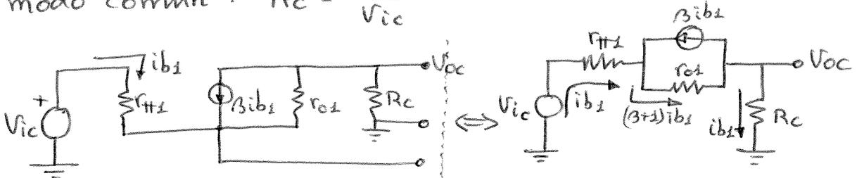
$$\left. \begin{aligned} V_{oc} &= i_{b1} \cdot R_c \\ V_{ic} &= i_{b1} [r_{\pi 1} + (\beta + 1)r_{o1} + R_c] \end{aligned} \right\} \boxed{A_c = \frac{V_{oc}}{V_{ic}} = \frac{R_c}{r_{\pi 1} + (\beta + 1)r_{o1} + R_c} = 0.002}$$
