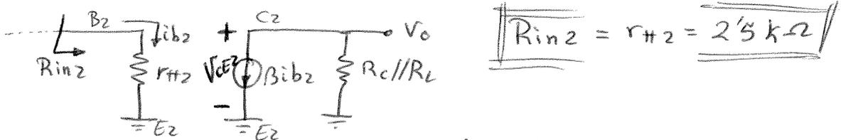
$$\underline{\underline{R_{in2} = r_{\pi 2} = 2.5 k\Omega}}$$
