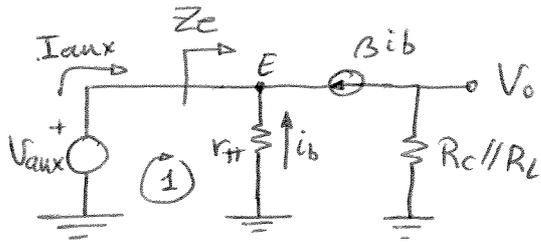
$$\begin{aligned} \text{malla 1: } V_{aux} &= -i_b r_{\pi} \\ \text{nudo E: } I_{aux} &= -i_b (\beta + 1) \end{aligned} \left. \vphantom{\begin{aligned} \text{malla 1: } V_{aux} &= -i_b r_{\pi} \\ \text{nudo E: } I_{aux} &= -i_b (\beta + 1) \end{aligned}} \right\} Z_e = \frac{V_{aux}}{I_{aux}} = \frac{+i_b r_{\pi}}{+i_b (\beta + 1)} = \frac{r_{\pi}}{\beta + 1} \approx \frac{r_{\pi}}{\beta} = 25 \Omega$$
