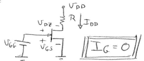
$V_{DZ} = V_{GG} + I_D R - V_{DD} = V_{GG} + k (V_{GS} - V_T)^2 R - V_{DD} = -6\text{ V}$  (correcto)
