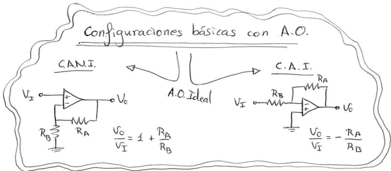
9)  $\frac{v_o}{v_i}$  ?? A.O. ideal  $\equiv$  lineal  $\begin{cases} I_+ = I_- = 0 \quad (Z_i \rightarrow \infty) \\ V_+ = V_- = v_i \end{cases}$
