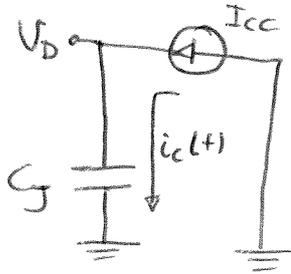
$$I_{cc} = i_c(t) = C_J \frac{\partial V_D(t)}{\partial t}$$
