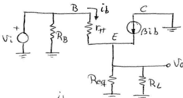
$r_{\pi} = \frac{\beta V_T}{I_C} = 5\text{ k}\Omega$
