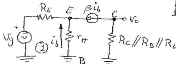
$$r_{\pi} = \frac{V_T}{I_B} = 1'52 \text{ k}\Omega$$
