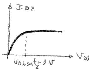
$V_{DS,sat1} = V_{GS} - V_{T1} = 2\text{ V}$
