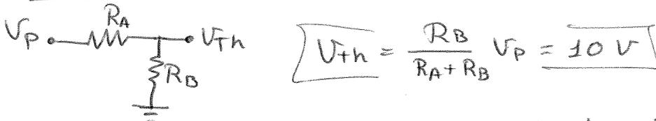
$$V_{Th} = \frac{R_B}{R_A + R_B} V_P = 10V$$
