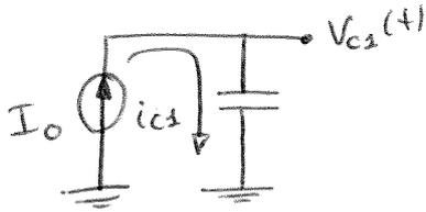
$$I_0 = i_{c2}(t) = C \frac{\partial V_{c2}(t)}{\partial t}$$
