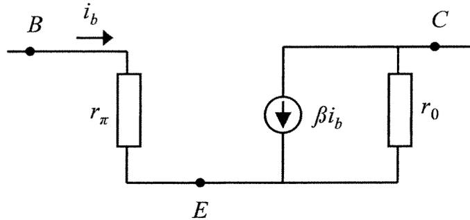
Donde:  $r_o = \left. \frac{\partial v_{CE}}{\partial i_C} \right|_Q = \frac{V_A}{I_{CQ}}$
