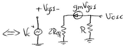
$$\begin{aligned} * V_{o1c} &= -g_m V_{gs1} R \\ * V_c - V_{gs1} - g_m V_{gs1} 2R_{eq} &= 0 \\ V_c &= V_{gs1} (1 + 2g_m R_{eq}) \\ V_{i1} &= 2V_{gs1} (1 + 2g_m R_{eq}) \end{aligned}$$
