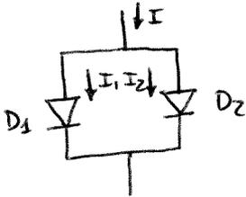
$$P_L = P_{L1} + P_{L2} = \delta I_1 + \delta I_2 = \delta (I_1 + I_2) = \delta I$$
