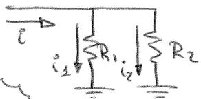
$$i_1 = \frac{R_2}{R_1 + R_2} \cdot i$$
