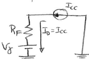
$$I_D = I_{CC} = 1 \text{ mA} > 0 \text{ (o.k.)}$$
