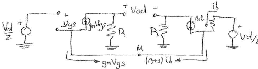
$$\left. \begin{array}{l} * \frac{V_d}{2} - V_{gs} - V_m = 0 \\ * -\frac{V_d}{2} - ib r_{\pi} - V_m = 0 \\ * g_m V_{gs} = -(\beta + 1) i_b \end{array} \right\} \begin{array}{l} \text{sistema} \\ \text{3 eqs} \\ \text{3 incóg.} \end{array}$$
