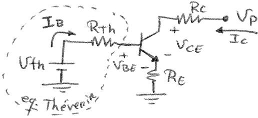
$$EE: V_{Th} - I_B R_{Th} - V_{BE} - I_E R_E = 0$$
