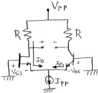
$$I_D = \kappa (V_{GS} - V_T)^2 = 2 \text{ m} (0,63 + 0,37)^2 = 2 \text{ mA}$$
