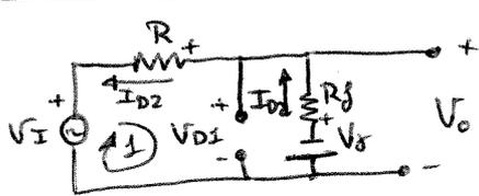
$$* V_o = -V_f - I_{D2} R_f = -V_f + R_f \frac{V_I + V_f}{R + R_f}$$
