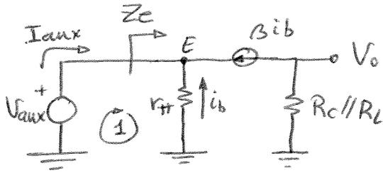
mall 1:  $V_{aux} = -i_b r_{\pi}$
