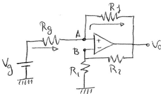
nudo A:  $\frac{V_G - V_+}{R_g} = \frac{V_+ - V_O}{R_f}$
