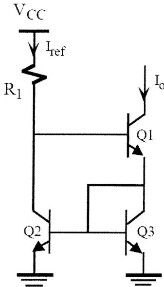
$$I_o \approx I_{ref} = \frac{V_{CC} - 2V_{BE}}{R_1}$$
