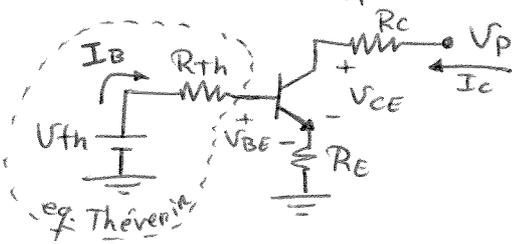
$$EE: V_{Th} - I_B R_{Th} - V_{BE} - I_E R_E = 0$$
