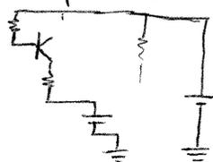
$$EE: V_{CE}^{sat} + I_E \cdot R_D + V_{BE} + I_B \cdot R_A - V_{CC} = 0$$
