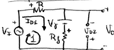
\*  $V_o = I_{D1} R_f + V_\gamma = R_f \frac{V_I - V_\gamma}{R + R_f} + V_\gamma = 0.0099 V_I + 0.495 = V_o$
