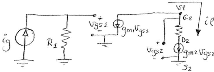
$$i_L = g_{m2} V_{gs2}$$
