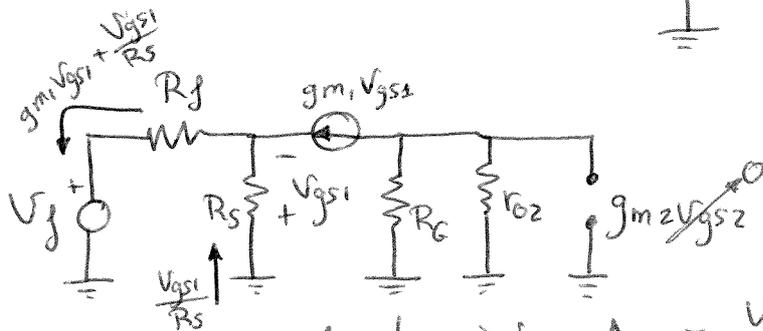
$$g_{m1} = 2k(V_{GS1} - V_{T1}) = 2.82 \text{ mS}$$
