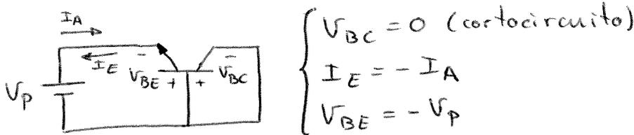
$$I_E = I_{ES} (e^{\frac{V_{BE}}{V_t}} - 1) - \alpha_R I_{CS} (e^{\frac{V_{BC}}{V_t}} - 1) \quad ; \quad \boxed{I_{ES} = \frac{-I_A}{e^{-\frac{V_P}{V_t}} - 1} = I_A = 10^{-6} \text{ A}}$$
