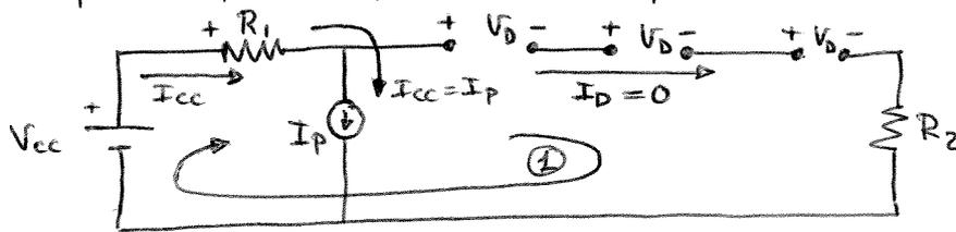
$$I_D = 0 \Rightarrow V_{R_2} = 0$$
