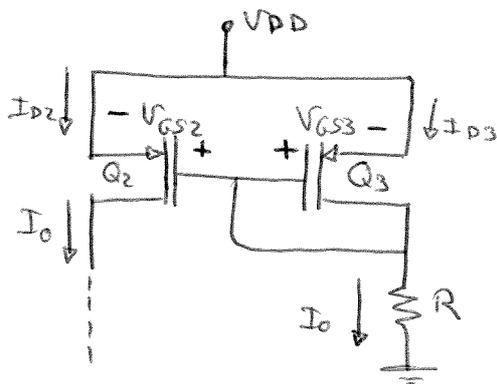
$$V_{GS2} = V_{GS3} \Rightarrow I_{D2} = I_{D3} = I_0$$
