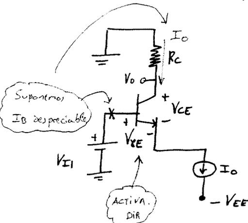
$$V_{CE} = V_{BE} - V_{I1} - I_0 \cdot R_C \geq V_{CE,sat}$$
