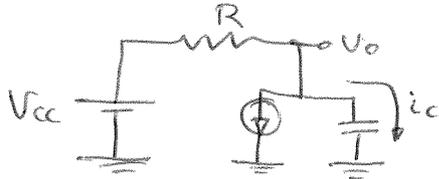
$$V_0(t) = V_{cc} - [I_L + i_c(t)]R =$$
