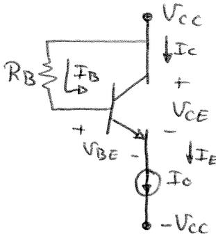
$I_E = I_0 = (\beta + 1) I_B \Rightarrow I_B = 4,98\mu\text{A} > 0$  (o.k.)
