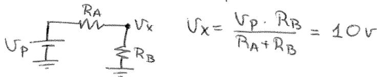
$$V_x = \frac{V_P \cdot R_B}{R_A + R_B} = 10 \text{ V}$$
