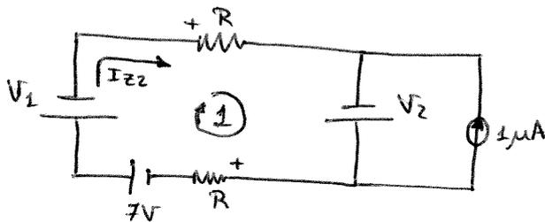
mallá 1:  $V_2 - V_1 - 2I_{Z2} \cdot R + 7 = 0$
