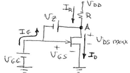
$V_{GS} = V_{GG} = -2V$  (ok)
