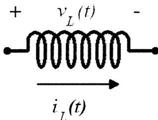
The diagram shows a coil with an arrow pointing to the right below it, labeled  $i_L(t)$ . Above the coil, there is a plus sign on the left and a minus sign on the right, with  $v_L(t)$  written between them.
