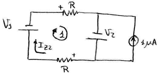
mallá 1:  $V_2 - V_1 - 2I_{Z2}R = 0$
