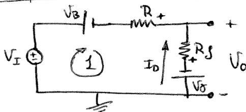
$$* V_o = -V_\gamma - R_f \cdot I_D = -V_\gamma - \frac{V_B - V_\gamma - V_I \cdot R_f}{R + R_f}$$
