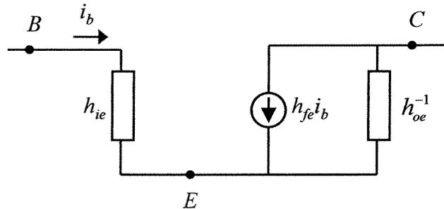
Donde:  $h_{ie} = r_\pi$        $h_{fe} = \beta$        $h_{oe}^{-1} = r_o$
