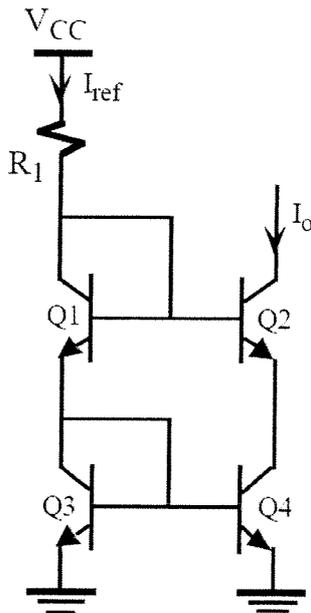
$$I_o \approx I_{ref} = \frac{V_{CC} - 2V_{BE}}{R_1}$$
