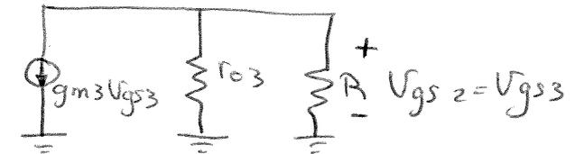
$$\frac{V_{gs3}}{i} = \frac{V_{gs3}}{g_{m3} V_{gs3}} = \frac{1}{g_{m3}}$$
