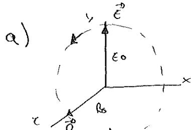
$$\begin{aligned}\vec{E} &= \begin{cases} E_x = 0 \\ E_y = E_0 \cos(\omega t - Kx) = E_0 \cos 2\pi f \left(t - \frac{x}{c}\right) \\ E_z = E_0 \sin(\omega t - Kx) = E_0 \sin 2\pi f \left(t - \frac{x}{c}\right) \end{cases} \\ \vec{B} &= \begin{cases} B_x = 0 \\ B_y = -B_0 \cos(\omega t - Kx) = -\frac{E_0}{c} \sin 2\pi f \left(t - \frac{x}{c}\right) \\ B_z = B_0 \cos(\omega t - Kx) = \frac{E_0}{c} \cos 2\pi f \left(t - \frac{x}{c}\right) \end{cases}\end{aligned}$$
