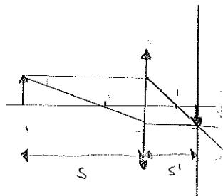
$$\begin{aligned} s + s' &= 0,18 \\ \frac{1}{s} + \frac{1}{s'} &= \frac{1}{0,04} \end{aligned} \quad \left\{ \begin{array}{l} s' = 0,18 - s \\ \frac{1}{s} + \frac{1}{s'} = 25 \end{array} \right.$$
