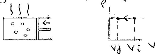
$$\omega = - \int_{V_i}^{V_f} P dV = - P_0 \int_{V_i}^{V_f} dV = - P_0 (V_f - V_i) = P_0 (V_i - V_f) > 0$$
