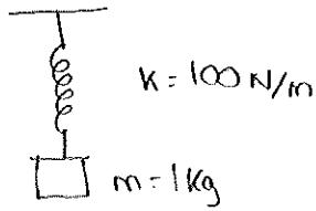
$$\text{a) } \omega_0 = \sqrt{\frac{K}{m}} = \sqrt{\frac{100}{1}} = 10 \text{ rad/s} \rightarrow T = \frac{2\pi}{\omega_0} = \frac{\pi}{5} \text{ s}$$
