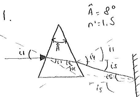
$$\left. \begin{array}{l} i_1 = \frac{\hat{A}}{2} = 4^\circ \\ i_2 = \arcsen\left(\frac{1}{n} \cdot \sin 4^\circ\right) = 2.66^\circ \end{array} \right\}$$
