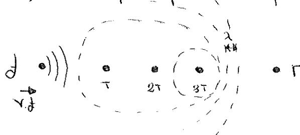
$$\Delta t_r = \frac{V}{\lambda_r} = \frac{V}{V_t - V_f T} = \frac{V}{V - V_f} \Delta t_f \Rightarrow \Delta t_r = \frac{V}{V + V_f} \Delta t_f \quad \left. \begin{array}{l} (-) \text{ se acerca} \\ (+) \text{ se aleja} \end{array} \right\}$$
