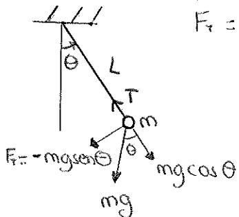
$$\begin{aligned} F_x &= -mg \sin \theta = ma = mL \ddot{\theta} = m L \frac{d^2\theta}{dt^2} \\ -mg \sin \theta &= m L \frac{d^2\theta}{dt^2} \\ L \frac{d^2\theta}{dt^2} + g \sin \theta &= 0 \end{aligned}$$
