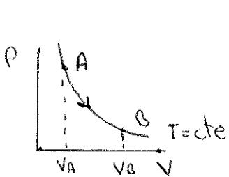
$$\Delta S = \int_A^B \frac{dQ}{T} = \int_{V_A}^{V_B} \frac{PdV}{T} = \int_{V_A}^{V_B} \frac{nRT}{V} \frac{dV}{T} = nR \ln \frac{V_B}{V_A}$$
