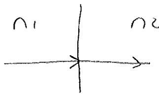
$$a) v_1 = \frac{c}{n_1} = \frac{3 \cdot 10^8}{2} = 1.5 \cdot 10^8 \text{ m/s}; v_2 = \frac{c}{n_2} = \frac{3 \cdot 10^8}{1.5} = 2 \cdot 10^8 \text{ m/s}$$
