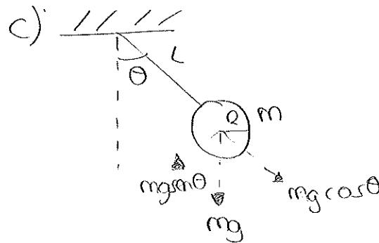
$$\left. \begin{array}{l} -mg(L+R)\sin\theta = \sum M \\ I \cdot \frac{d^2\theta}{dt^2} = I\alpha \end{array} \right\} \begin{array}{l} I \frac{d^2\theta}{dt^2} + mg(L+R)\sin\theta = 0 \\ \end{array}$$
