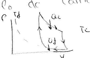
$$\epsilon = \frac{\omega}{Q_c} = \frac{Q_c - Q_f}{Q_c} = 1 - \frac{Q_f}{Q_c} = 1 - \frac{nRT_f \ln \frac{V_c}{V_f}}{nRT_c \ln \frac{V_f}{V_c}}$$
