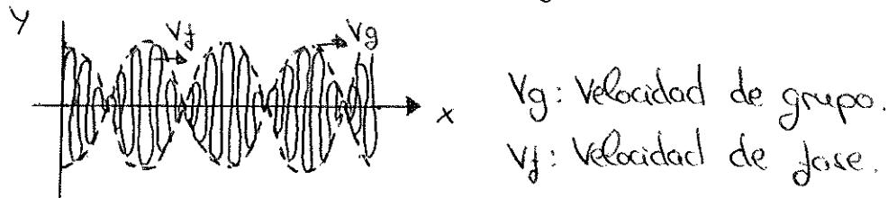
$$V_g = \frac{\omega - \omega'}{k - k'} = \frac{d\omega}{dk} = V + \frac{k dV}{dk}$$
