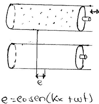
$$P = F \cdot V = \dots = \rho_0 V A \omega^2 e_0^2 \cos^2(kx + wt)$$
