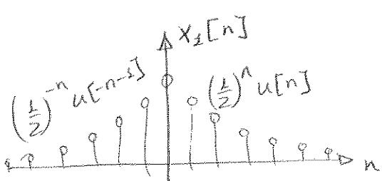
$$X_1(e^{j\omega}) = \frac{1}{1 - \frac{1}{2} e^{j\omega}} + \frac{\frac{1}{2} e^{j\omega}}{1 - \frac{1}{2} e^{j\omega}}$$
