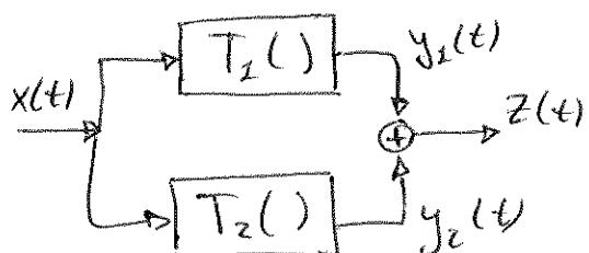
$$z(t) = y_1(t) + y_2(t) = T_1(x(t)) + T_2(x(t))$$
