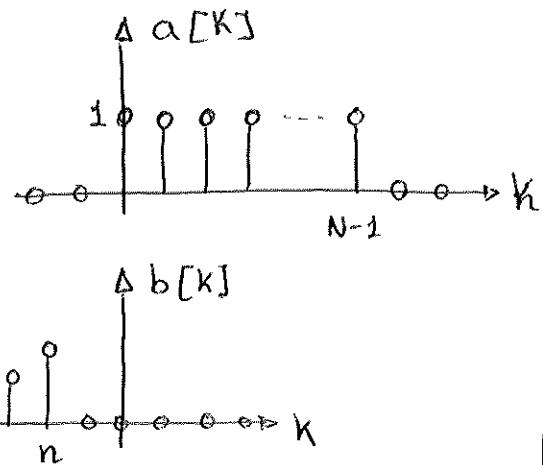
$$\left. \begin{array}{l} n < 0 : c[n] = 0 \\ 0 \leq n \leq N-1 : c[n] = \sum_{k=0}^n \beta^{n-k} = \\ \quad = \beta^n \cdot \frac{1 - \beta^{n+1}}{1 - \beta} \\ n > N-1 : c[n] = \sum_{k=0}^{N-1} \beta^{n-k} = \\ \quad = \beta^n \cdot \frac{1 - \beta^{-N}}{1 - \beta} \end{array} \right\}$$
