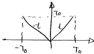
$$X(j\omega) = \int_{-\infty}^{+\infty} x(t) e^{-j\omega t} dt = - \int_{-T_0}^0 t e^{-j\omega t} dt + \int_0^{T_0} t e^{-j\omega t} dt$$
