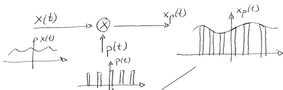
$$X_p(j\omega) = \sum a_k X(j(\omega - k\omega_s)), \quad a_k = \frac{P_p(j\omega)}{\pi} \Big|_{\omega = k\omega_s}$$
