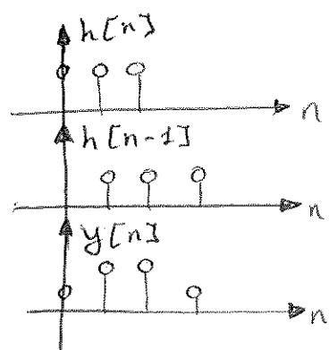
$$\text{Ej: } \left. \begin{array}{l} x[n] = \alpha^n u[n], \alpha \in (0, 1) \\ h[n] = u[n] \end{array} \right\} \quad \begin{array}{l} y[n] = x[n] * h[n] \\ y[n] = \sum_{k=-\infty}^{+\infty} x[k] \cdot h[n-k] \end{array}$$
