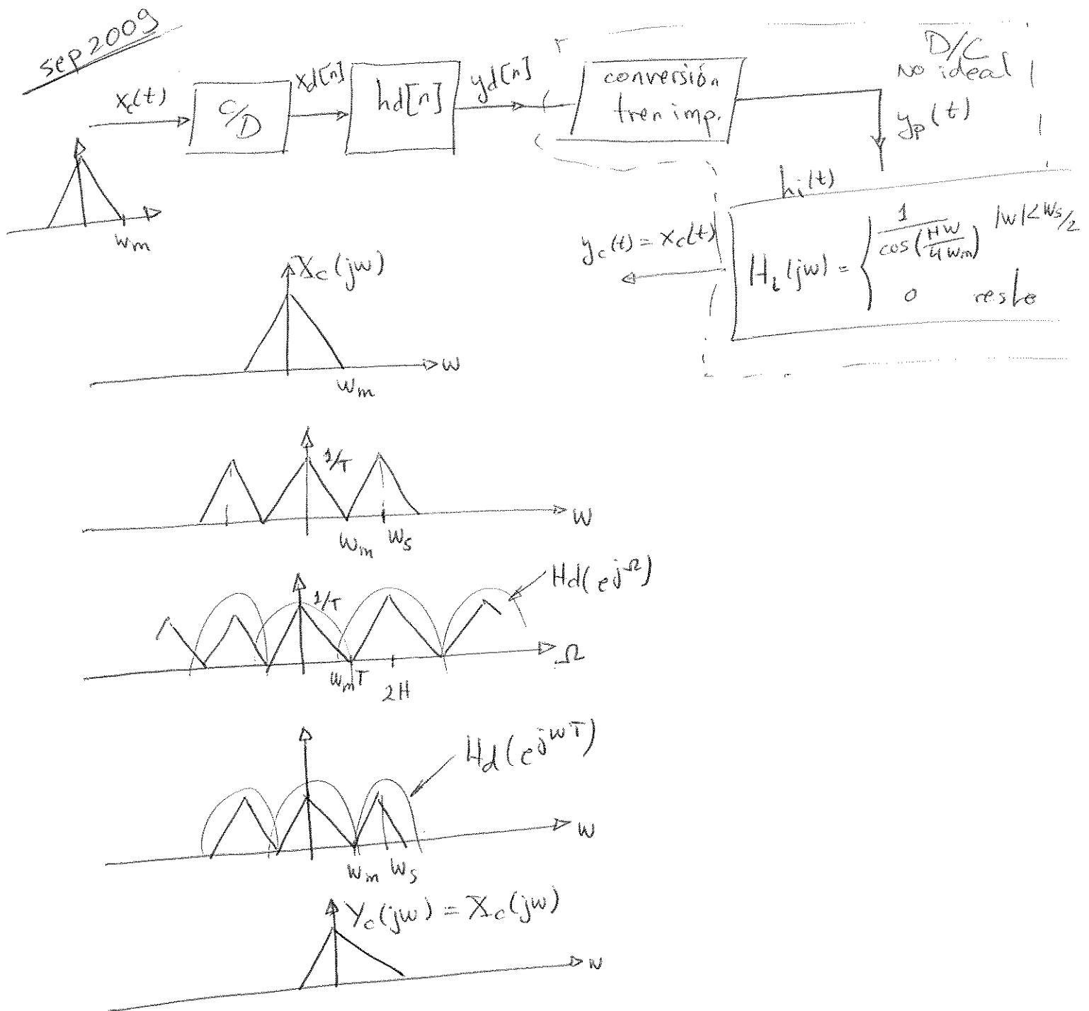
$$H_d(e^{j\omega T}) \cdot H_i(j\omega) = \begin{cases} T, & |\omega| < \omega_s/2 \\ 0, & \text{resto} \end{cases}$$
