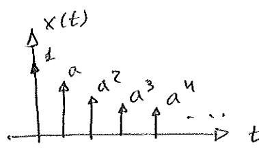
$$\begin{aligned} X(j\omega) &= \sum_{k=0}^{\infty} a^k \text{TF}(\delta(t - kT)) \\ &= \sum_{k=0}^{\infty} a^k e^{-j\omega kT} = \sum_{k=0}^{\infty} (a \cdot e^{-j\omega T})^k \\ &= \frac{1}{1 - a e^{-j\omega T}} \end{aligned}$$
