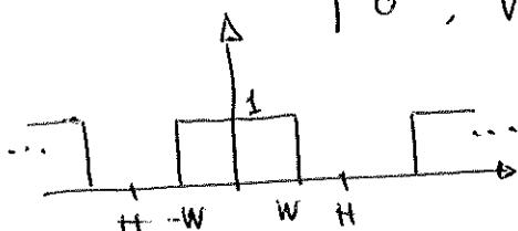
$$x[n] = \frac{1}{2\pi} \int_{-\pi}^{\pi} X(e^{j\omega}) e^{j\omega n} d\omega = \frac{1}{2\pi} \int_{-W}^W e^{j\omega n} d\omega$$
