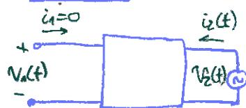
$$\begin{aligned} v_1(t) &= 0.5\cos t \Rightarrow E_1 = 0.5 \\ v_2(t) &= \cos t \Rightarrow E_2 = 1 \\ i_2(t) &= 3\sin t \Rightarrow I_2 = -3j \\ i_2(t) &= 3\sin t = 3\cos(t - \frac{\pi}{2}) \\ I_2 &= 3e^{-j\frac{\pi}{2}} = -3j \end{aligned}$$
