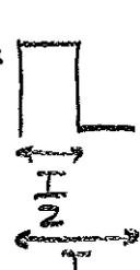
$$X_{\text{DC}} = P_0 X_{\text{DC}|'0''} + P_1 X_{\text{DC}|'1''} = \frac{A_{\text{Tx}}}{4} \rightarrow \boxed{P_{\text{DC}} = X_{\text{DC}}^2 = \frac{A_{\text{Tx}}^2}{16} = 19,8 \text{ mW}}$$
